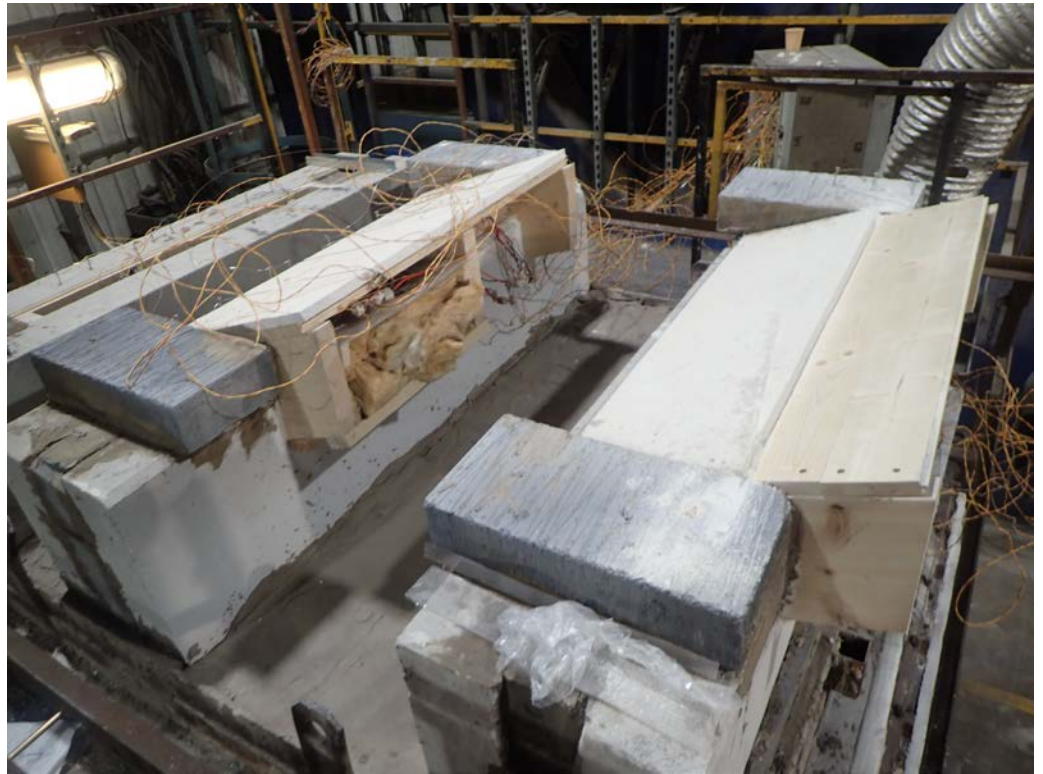
The unexposed face of the floor construction at the start of the test
