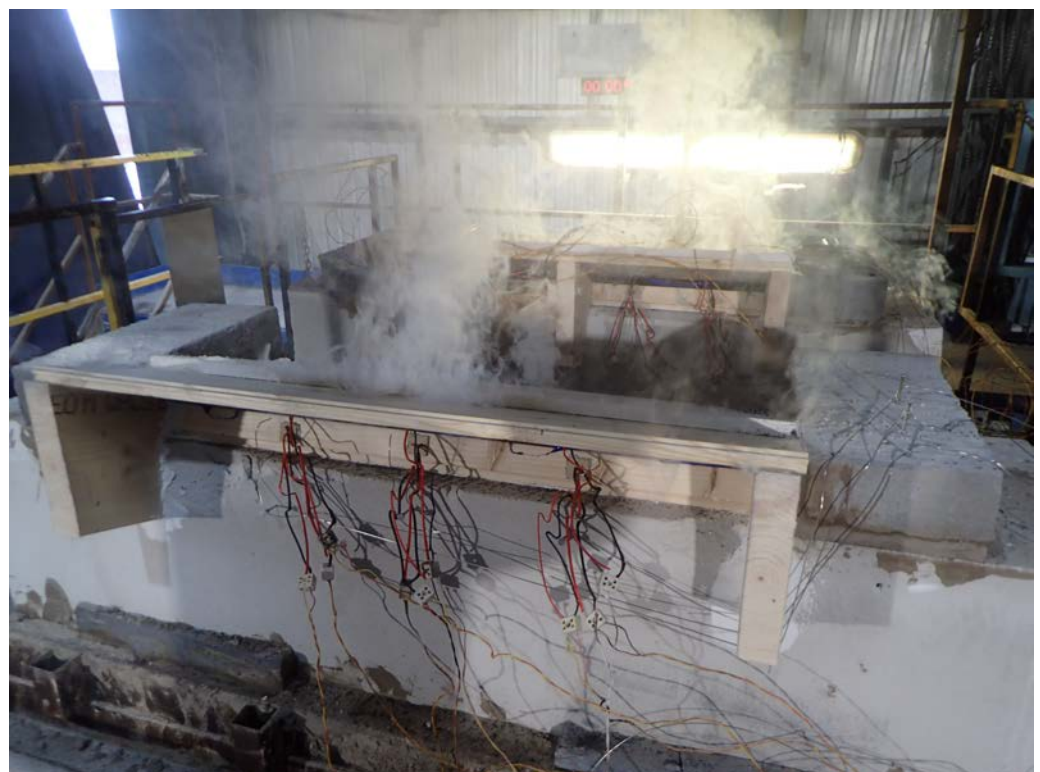
The unexposed face of the floor construction after a test duration of 60 minutes
