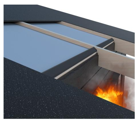
Intumescent material expands when exposed to external heat, sealing the roof cavity and preventing the spread of the flames.
